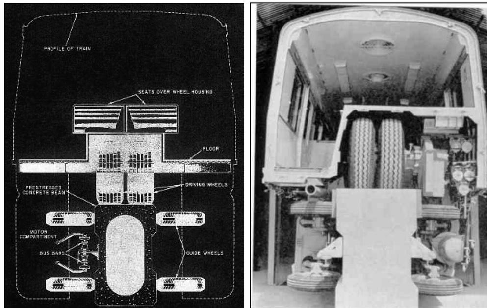
Figure 2.11—Cross-section of Alweg monorail showing seats over wheel housing, Source: The Alweg Archives
