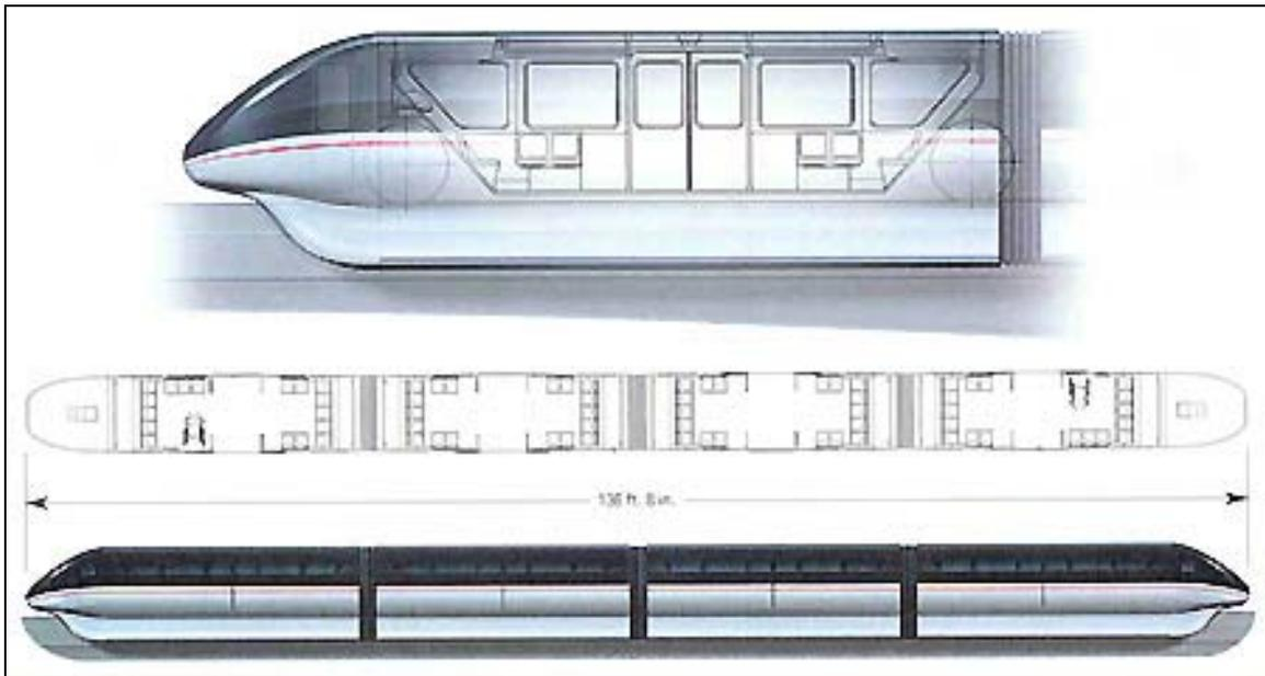
Figure 2.16—Bombardier Mark VI (Las Vegas Model), sleek and stunning but with no passenger-walk through between cars. Source: Las Vegas Monorail Company
