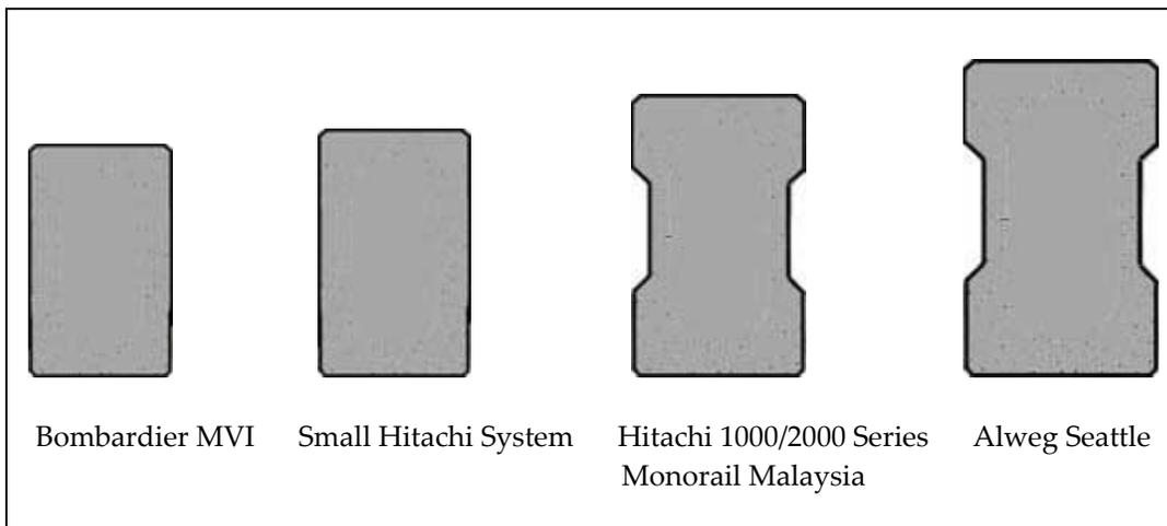
Figure 2.1—Relative Comparison of Guideway Beam Cross-sections. Source: The Monorail Society
