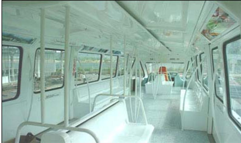
Figure 2.18—Monorail Malaysia train interior. The nearly ten foot width creates a sense of spaciousness despite the relatively low ceiling. Source: Elevated Transportation Company.
