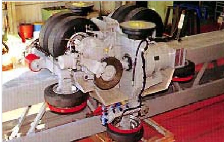
Figure 1.6—Two axle Rubber tired Hitachi monorail bogie. Source: Hitachi
