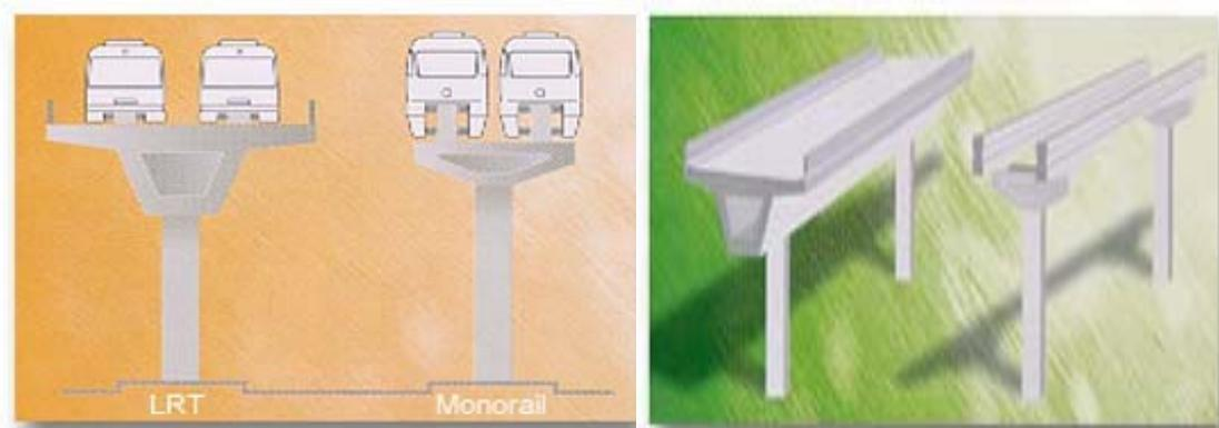
Figure 2.3—Comparison of large-type straddle-monorail with light rail aeriels. Source: Monorail Malaysia.
